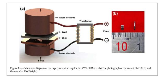
parts and micro patterns with high quality. In contrast with the capacitive discharge forming, the electric current stands at a constant value during the RWF, making it a convenient and controllable method for the millisecond thermoplastic forming of BMGs.
