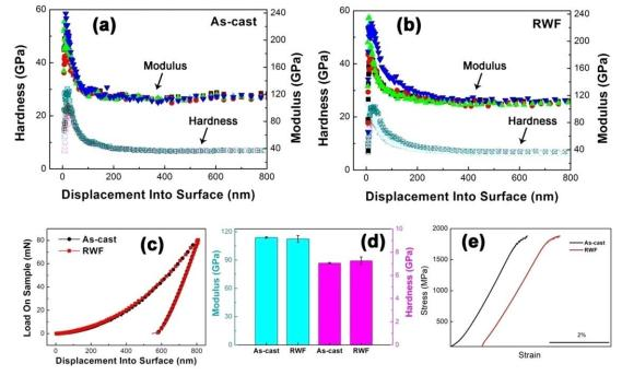
**Figure 4.** (a) and (b) present the hardness and modulus of the as-cast and RWF samples change along with the displacement into surface. (c) compares the load–depth curves of the as-cast and RWF samples. (d) plots the modulus and hardness of the as-cast and the RWF sample. (e) Mechanical properties of the as-cast and RWF samples.
